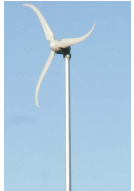
This 1.7 kilowatt wind turbine on the Hastings Campus will help students learn about alternate energy sources.
